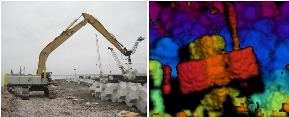
Figure 8. Excavator with Echoscope frame attached to the boom (left); example of Echoscope image (right)
