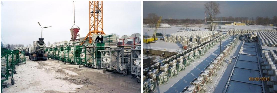
Figure 7. Xbloc moulds with polystyrene insulation for winter production
